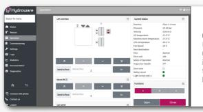
Use the operations menu to quickly see the status of the lift. Check where the lift is located in the shaft, if the safety circuit is open or closed or quickly access data such as machine room temperature, pressure, velocity, door zones and more. You can hold the doors in position or make the lift non-callable.
